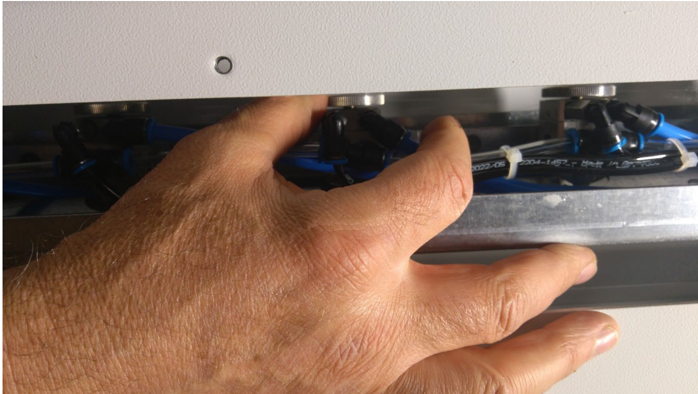
Manual nozzle adjustment by knurled wheel
